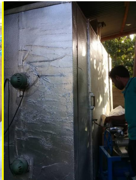
Photo Credit CRS-TL: Big dehydration machine has dried products over 500 kg with large electrical consumption
